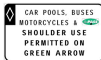
Figure MN-5. Static sign for dynamic shoulder lane.
