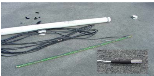
Figure AK-1. Thermistor string and temperature probe casing.
